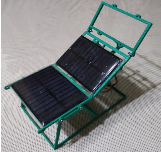
Figure 19 : Fixed and Tilting PV Panel Setup
