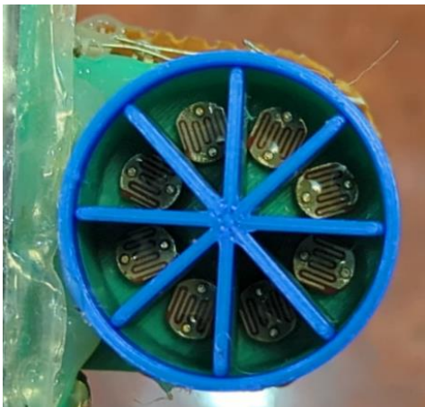
Figure 24 : LDRs Arrangement Module
