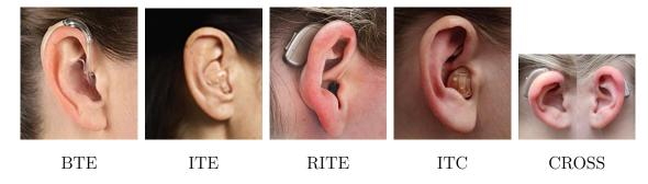
Figure 2.1: Different Types of Hearing Aids: BTE, ITE, RITE, ITC, and CROSS
