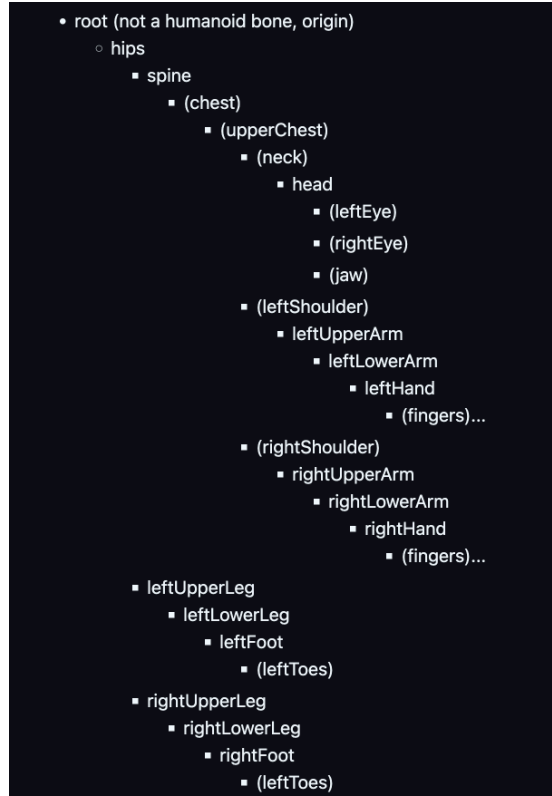
Figure 8: Rig keypoints structure from VRM Humonoid Spec
