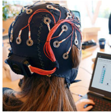
Figure 3.3: Emotive EPOC Flex Headset plugged in
