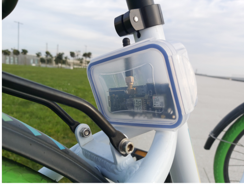
Figure 4: LoRa Tracking device on BIRA bicycle (Torres et al., 2021)
