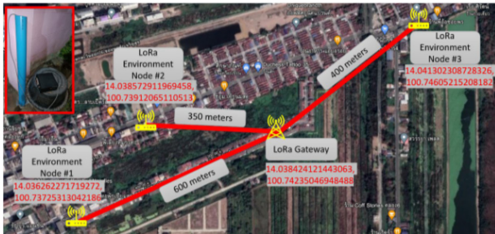
Figure 3: LoRa network for agriculture Chanwattanapong et al., 2021
