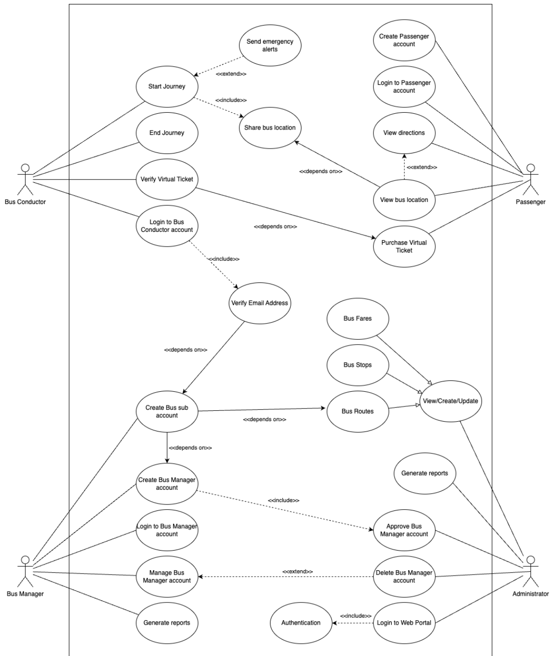
Figure 3.2: High level Use Case diagram
