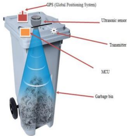
Figure 9: Prototype design of garbage bin
