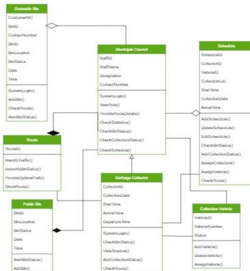
Figure 4: Class Diagram for the proposed system
