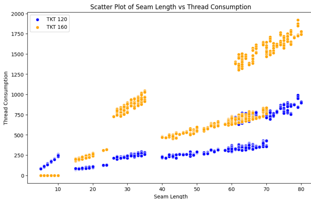
Figure 4.3 Influence of Seam Length on the thread consumption
