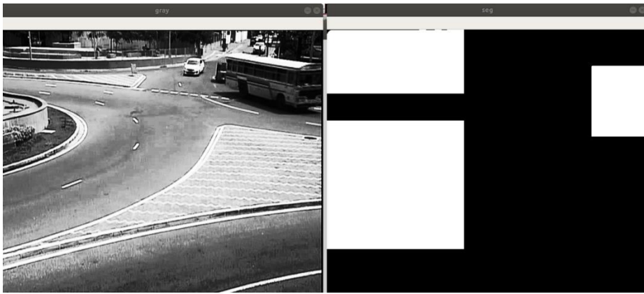
Figure 6. Selected rectangular region in video frame to avoid multiple detections of a vehicle
