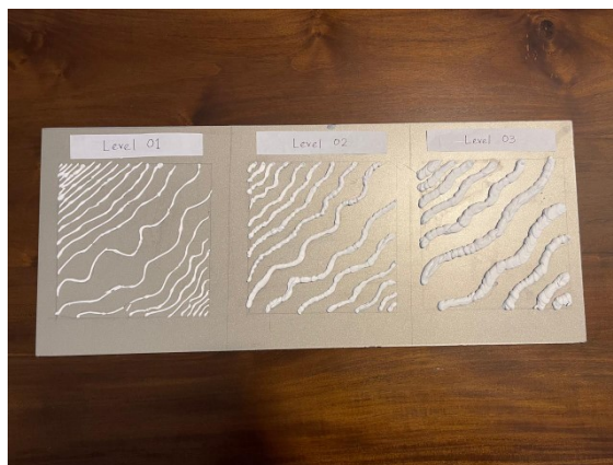
Figure 3.2: Embossed lines with various width and thickness were presented
