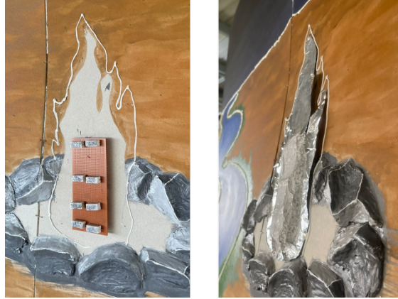
Figure 4.6: Actuator for Heat Stimulation Using 9 Parallelly Powered Resistors Covered with Heat Conductive Aluminum to Distribute Heat in the Shape of the Fire
