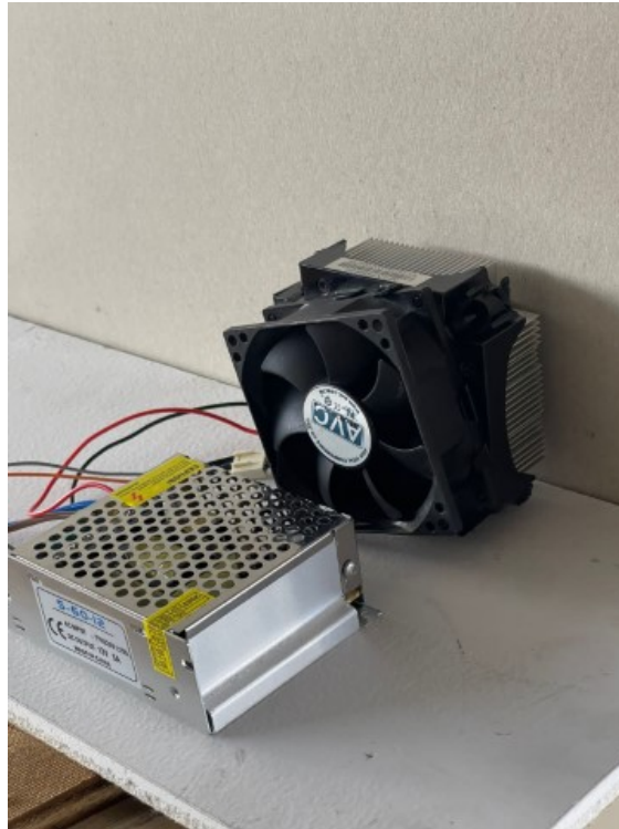
Figure 4.10: Actuator for Cold Stimulation Using a Peltier Module and a Case Fan Integrated into the Painting
