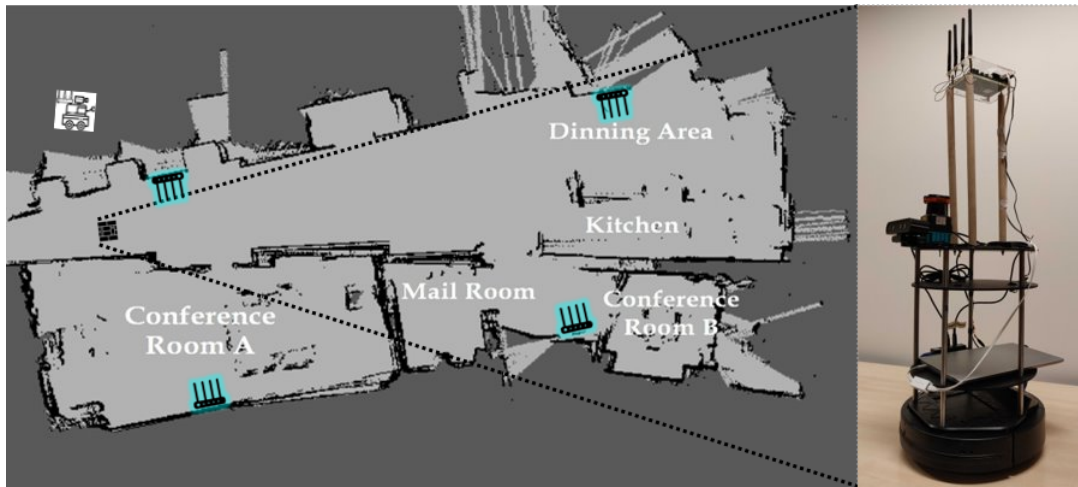
Figure 3.1: MapFind (right) is an autonomous robotics platform that creates a map (left) for indoor navigation and collects ground truth labelled CSI data for neural network training.
