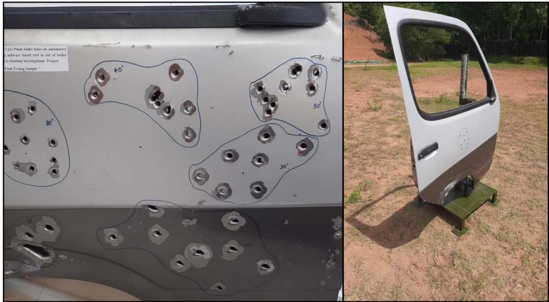
Figure 35. Captured Firing Data Samples Using a Van Door Made of 1 mm Zinc Coated Sheet Metal
