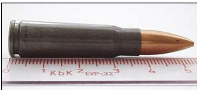
Figure 4. A steel-Cased 7.62 x 39 mm Ammunition (“7.62 x 39 mm,” 2022, p. 62)
