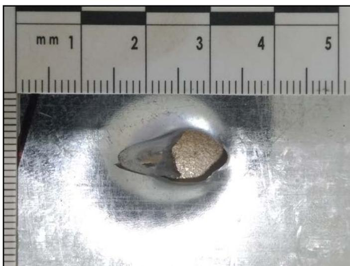
Figure 10. A Digitized Firing Data Sample from  $30^\circ$  Incident Angle by Placing a Forensic Ruler Close to the Bullet Impact Mark
