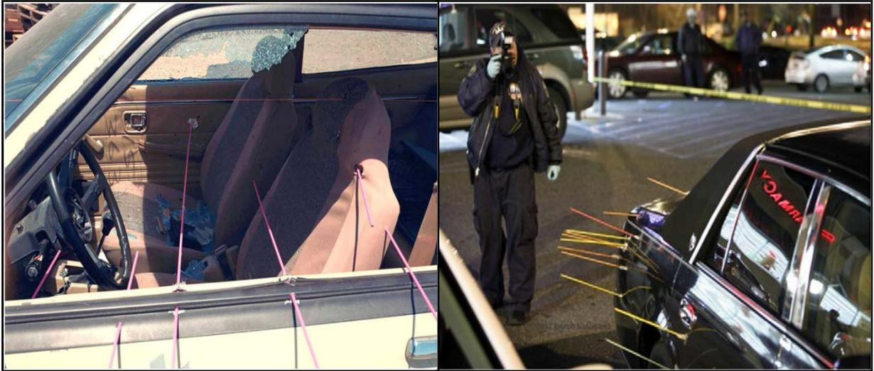
Figure 2. Using the Trajectory Rod Method to Understand the Shooter's Location
