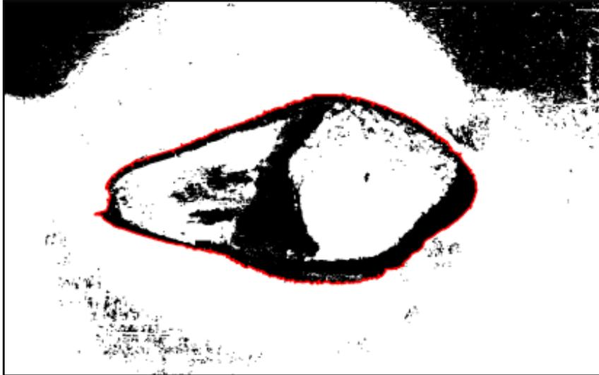
Figure 29. Identified Largest Contour (in Red Colour) Enclosing the Bullet Impact Mark
