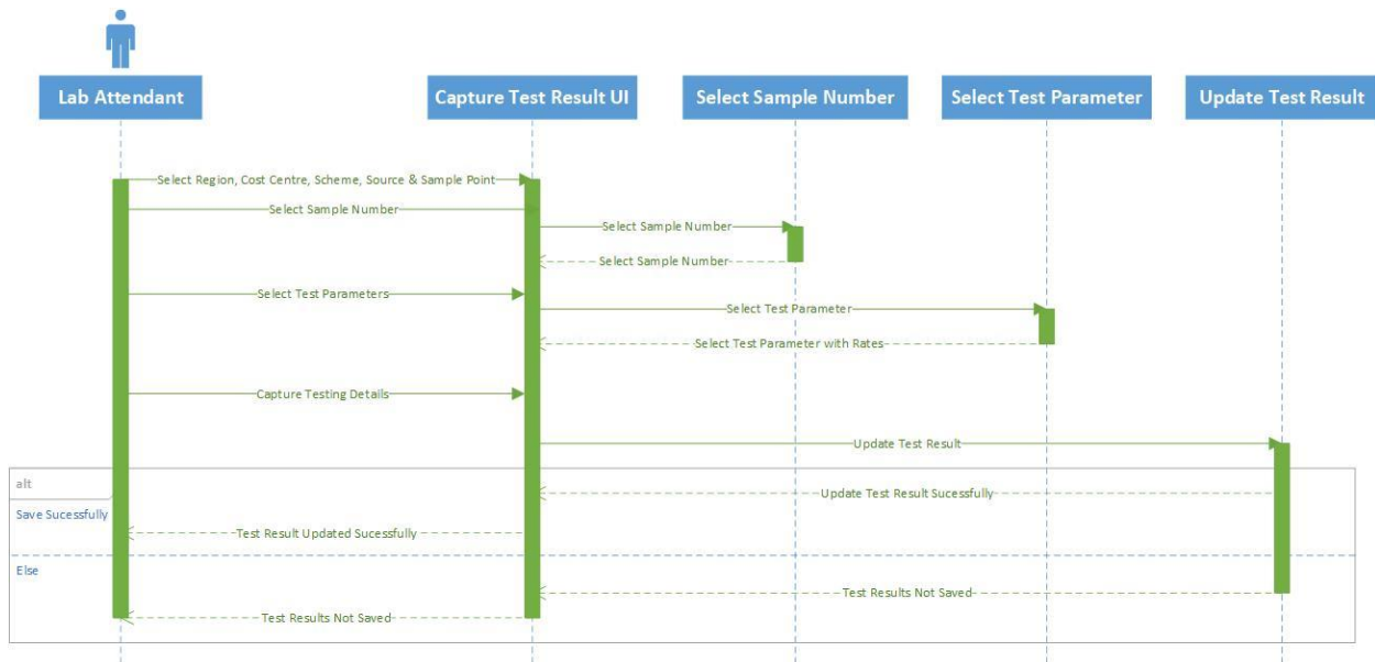
Figure 3.10: Update Test Result Sequence Diagram
