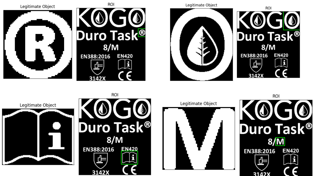
Figure 3.25: Define ROI around the Inspection object
