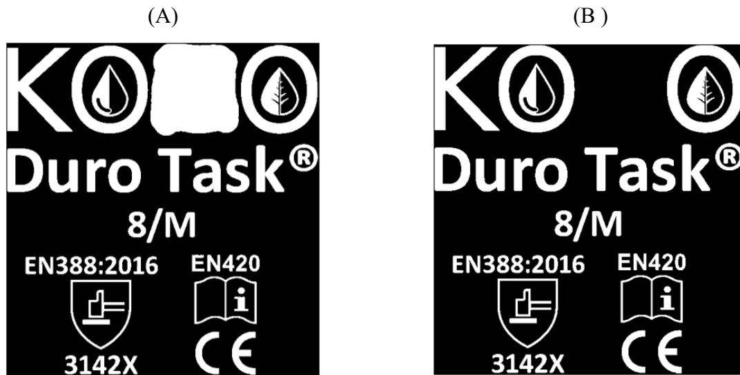
Figure 4.6: High-level object defects; (A) object missing due to inkblot, (B) object missing
