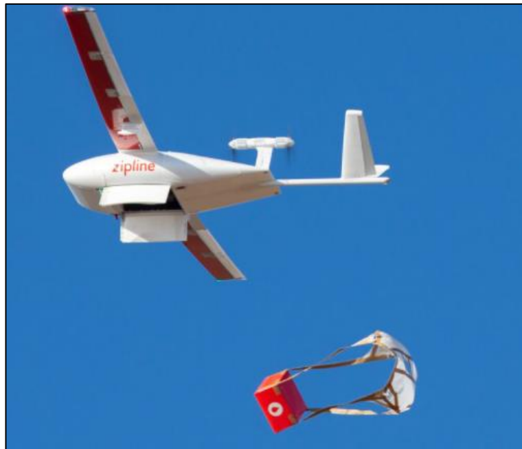
Figure 2: Fixed-wing UAV used to deliver medical supplies
