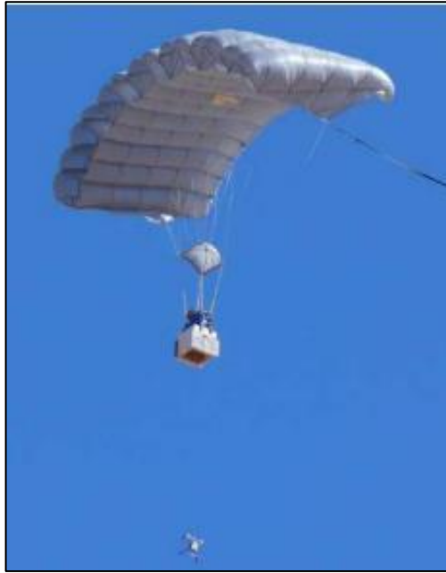
Figure 10: Autonomous airdrop using JPADS system
