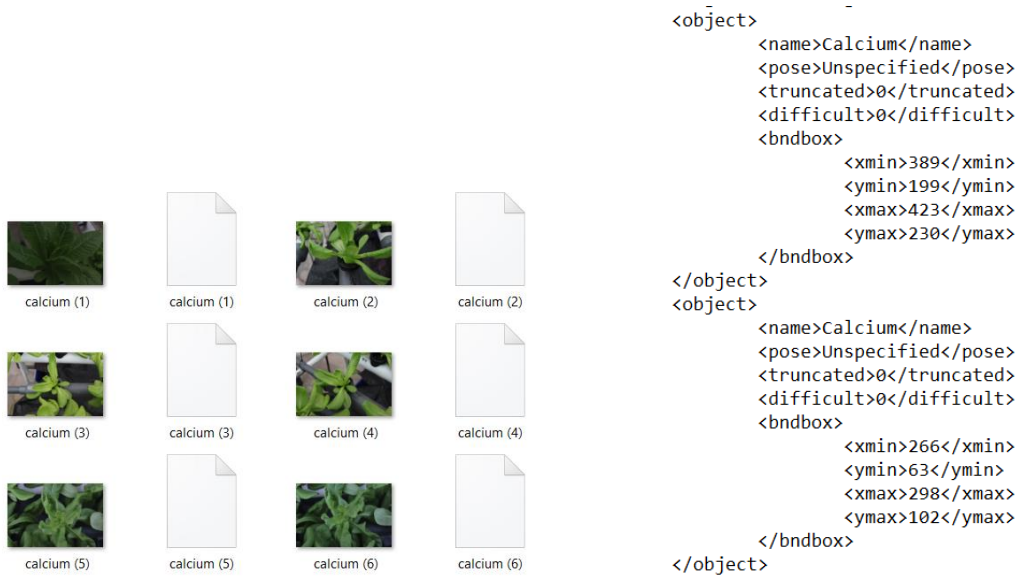
Figure 3.8: Left - annotation text files per each image with the same name as image. Right - Annotation file contains the coordinates of each bounding box of the image against the class name
