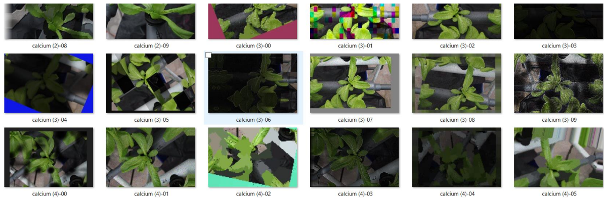
Figure 3.9: Augmented images using bounding-box-augmentation [92] based on imgaug [91] python library. Each image generates maximum of 10 augmentations according to the above techniques
