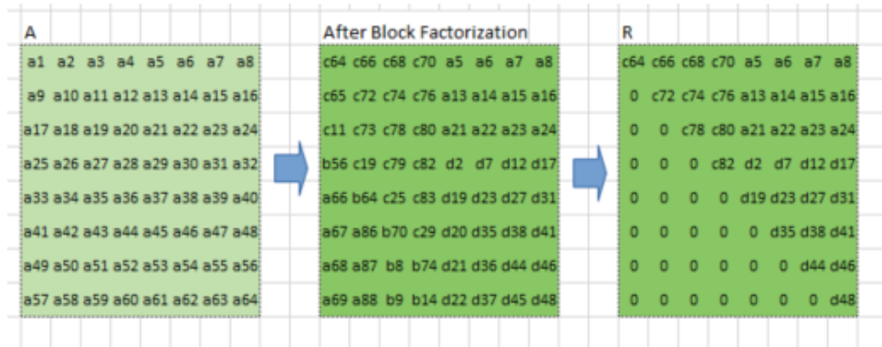
Figure 4.19 Remove the elements below the diagonal in R matrix
