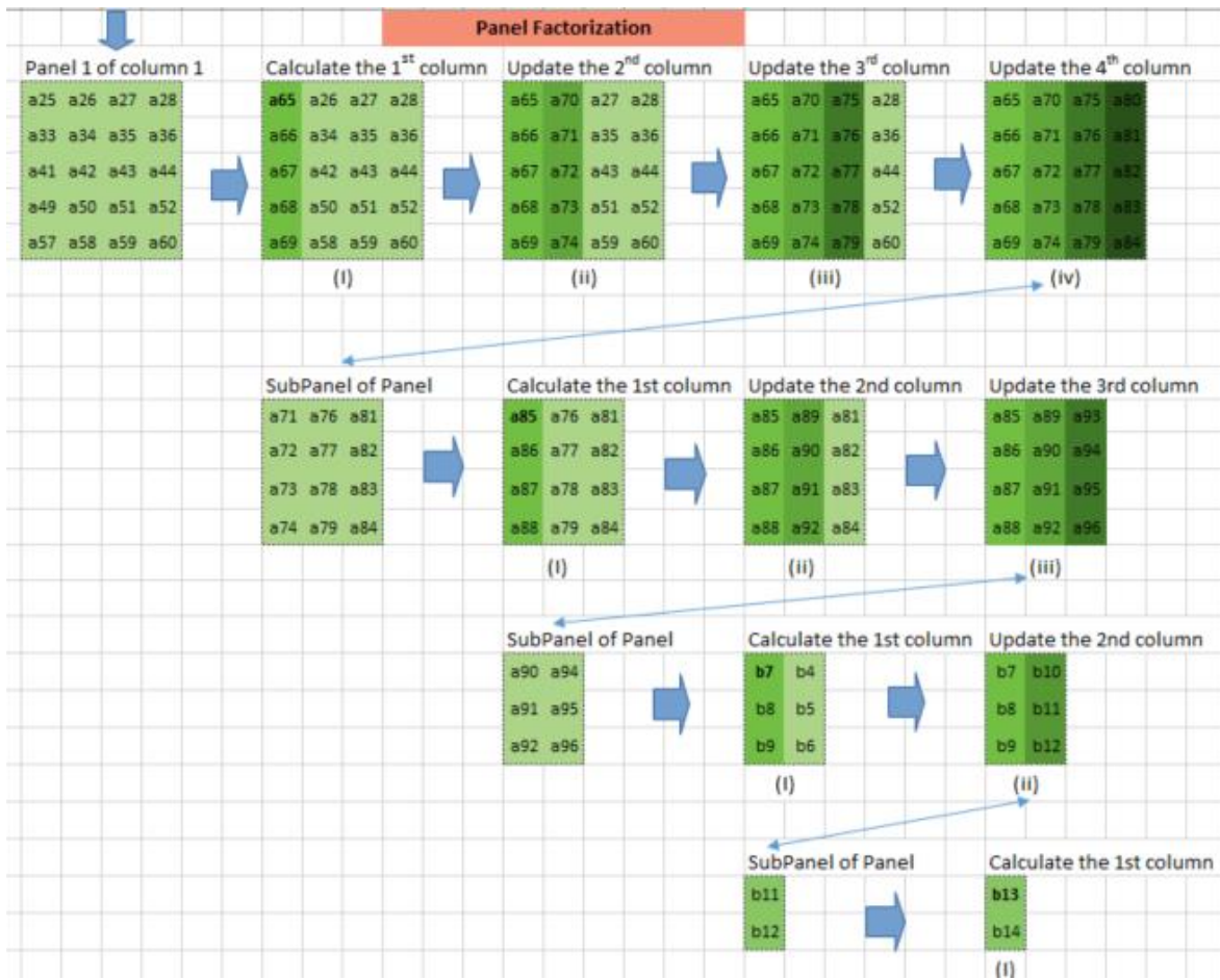
Figure 4.15 Panel factorization of panel 1 of column 1
