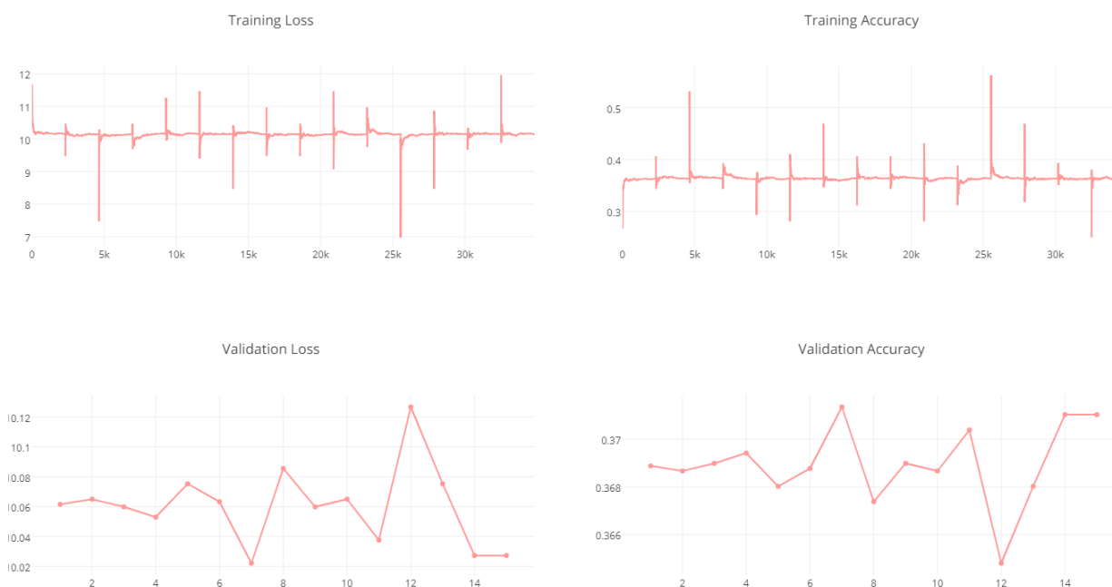
Fig. 32. Performance of activation function Tanh in Convolutional layers, Dense 1 Relu and Dense 2 Softmax of the model in Figure 21
