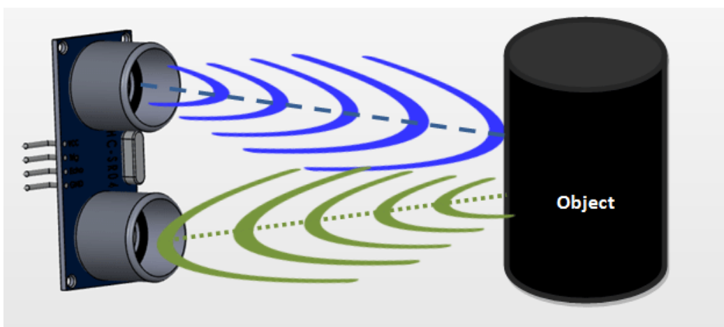
Figure 3.6 behavior of ultrasonic sensor
