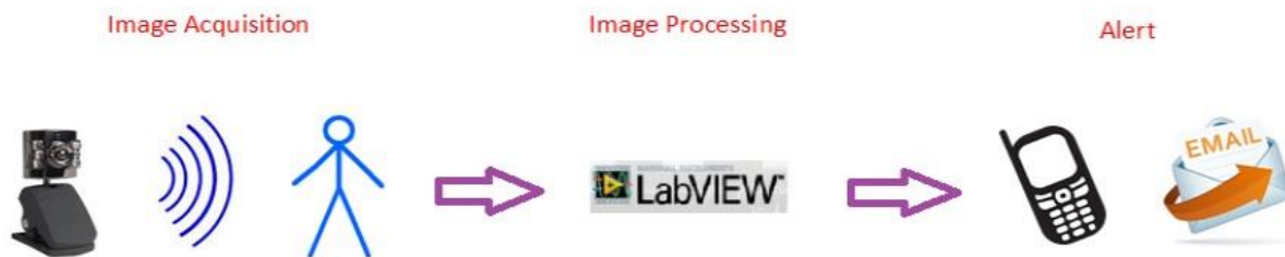
Figure 2.1 : A.Chiang, J.Chu and S.Su - proposed system of the Intruder Detection [ 1 , fig. 1]
