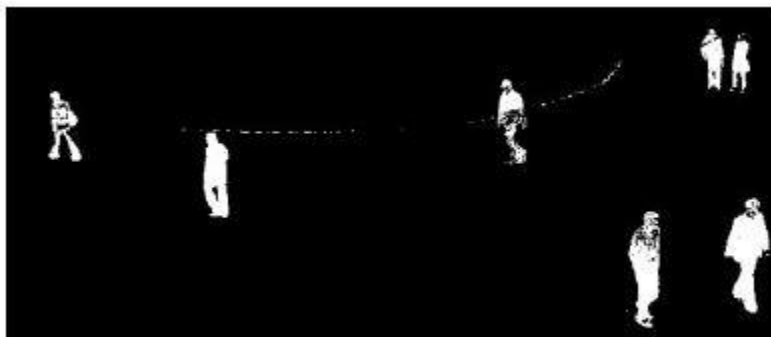
Figure 4.4 : Results of Background SubtractorGMG [ 7 , fig. 4 ]
