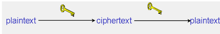
Figure 2.2: Secret Key (symmetric) cryptography uses single key [1]
