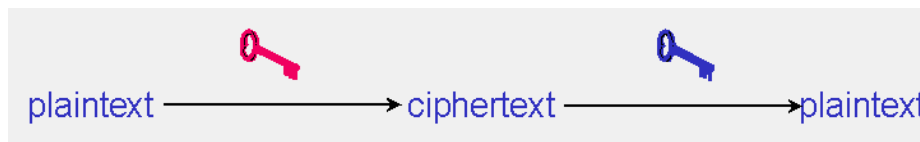
Figure 2.3: Public Key (asymmetric) cryptography uses two keys [1]
