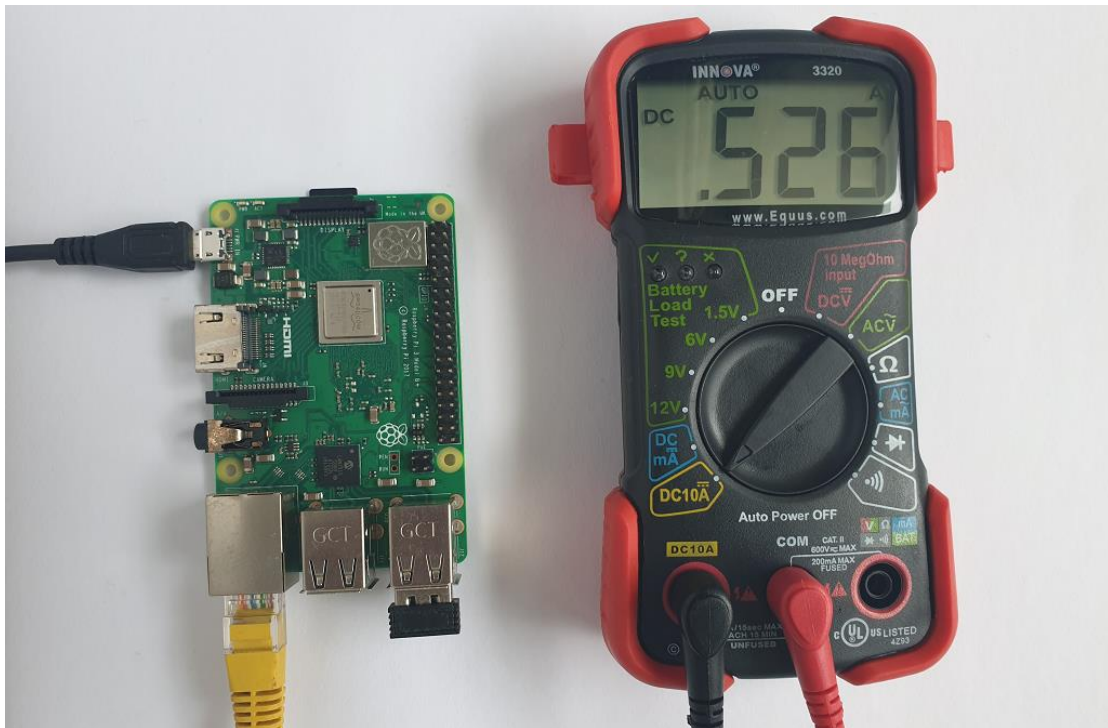
Figure 5.12: Aggregator Device Power Consumption Measurement Setup
