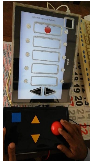
Figure 8.2 : A participant using Button Tactile Ballot
