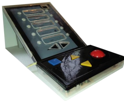
Figure 5.7 : Button Tactile Ballot and Touch Tactile Ballot (Side View)
