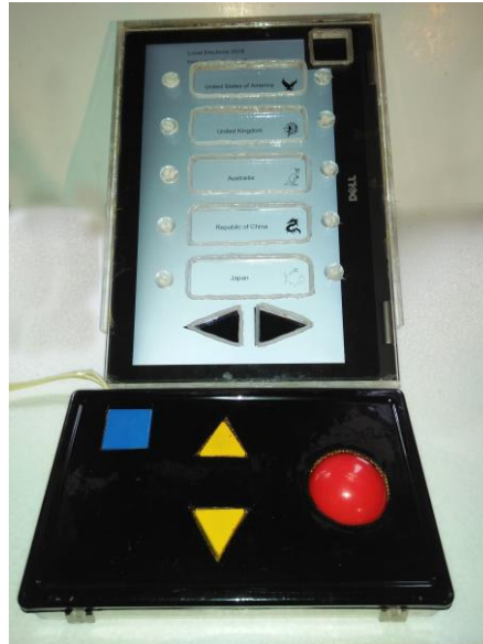
Figure 5.6 : Button Tactile Ballot and Touch Tactile Ballot (Front View)
