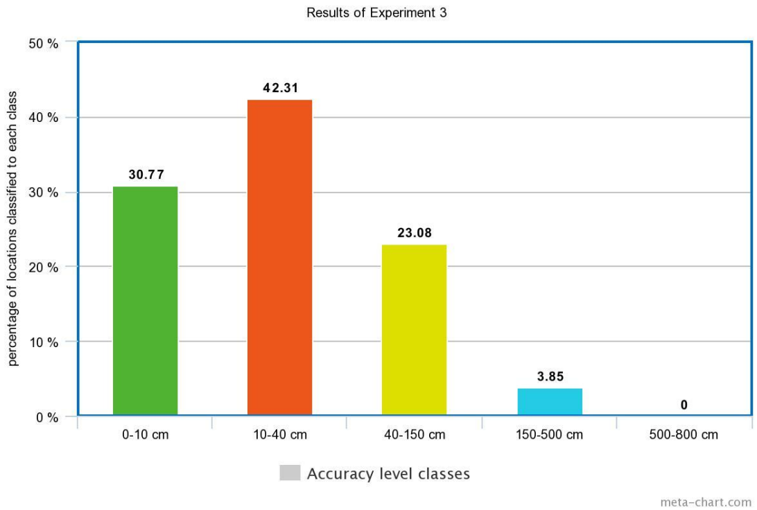
Figure 5.19: Graphical representation of the summary of results obtained by comparing data obtained using RTK device against data obtained in Experiment 3.
