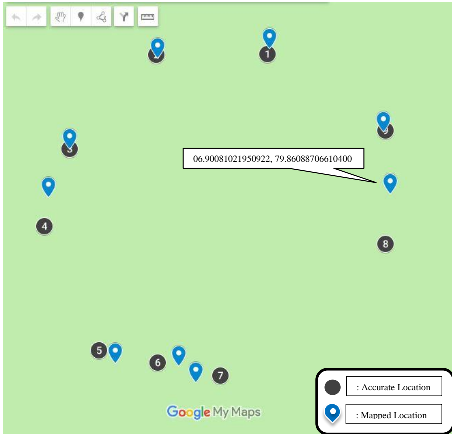
Figure 5.12: Mapping of position localization data of RTK device against data obtained in Experiment 2 for locations that are 650cm away from the object.
