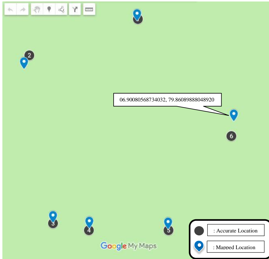
Figure 5.13: Mapping of position localization data of RTK device against data obtained in Experiment 2 for locations that are 750cm away from the object.
