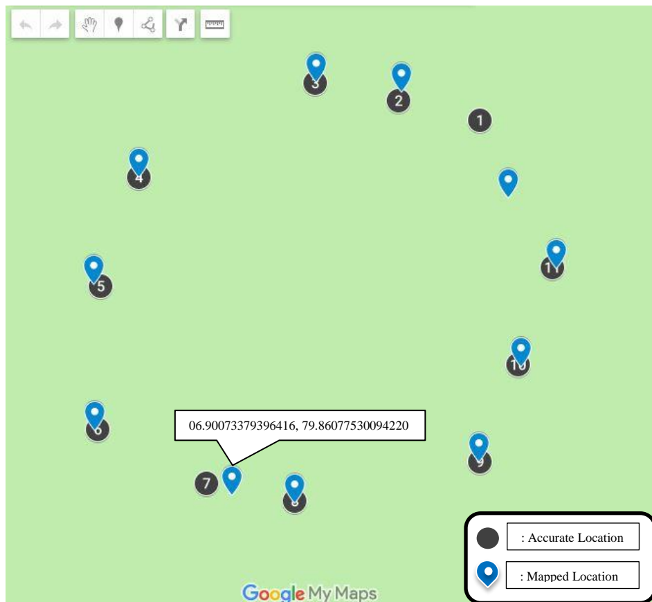
Figure 5.16: Mapping of position localization data of RTK device against data obtained in Experiment 3 for locations that are 550cm away from the object.
