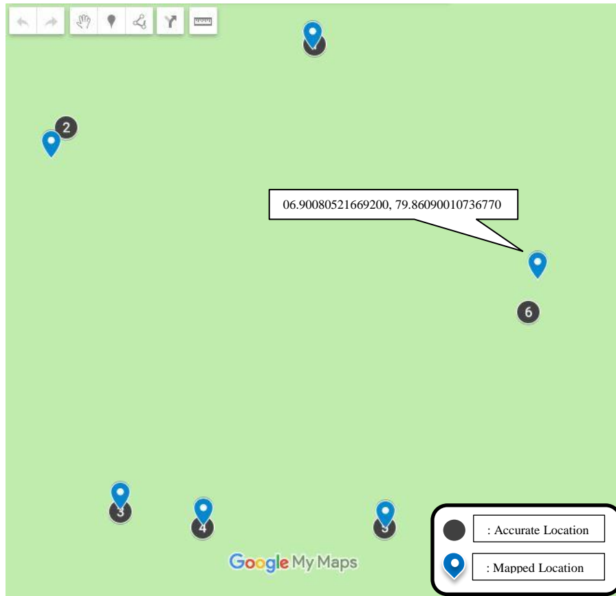
Figure 5.18: Mapping of position localization data of RTK device against data obtained in Experiment 3 for locations that are 750cm away from the object.
