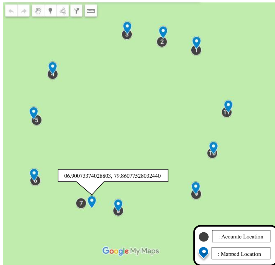
Figure 5.6: Mapping of position localization data of RTK device against data obtained in Experiment 1 for locations that are 550cm away from the object.
