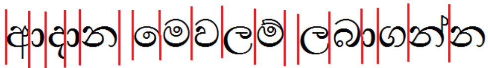
Figure 3.2: Vertical segmentation of characters
