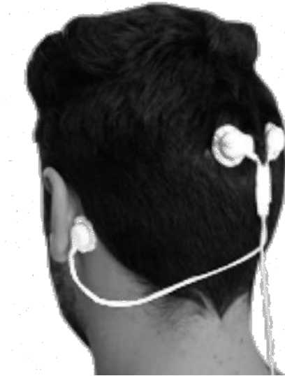
Figure 4.3 Connecting BITalino 3 electrode cable for EEG signal acquisition
