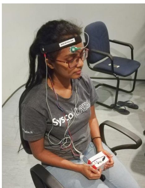
Figure 5.9 Detail of the way the band is put on for female users
