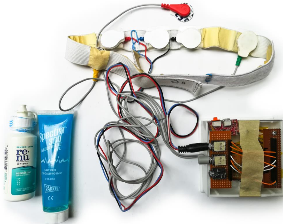
Figure 4.7 The custom-made EEG band (Version 1.0) connected to the device and the electrode gel and solution (left)
