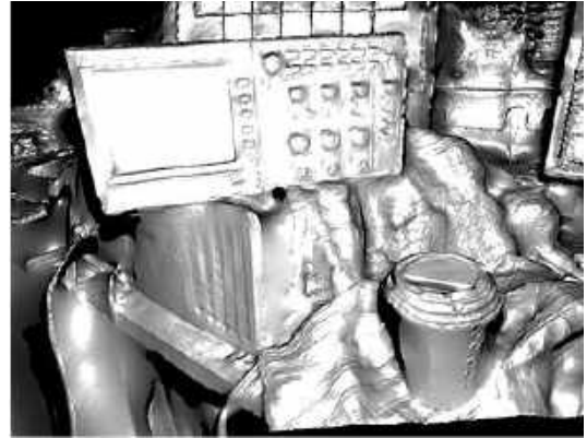
(b) The dense map generated by the DTAM system. All points on the surface are part of the map
