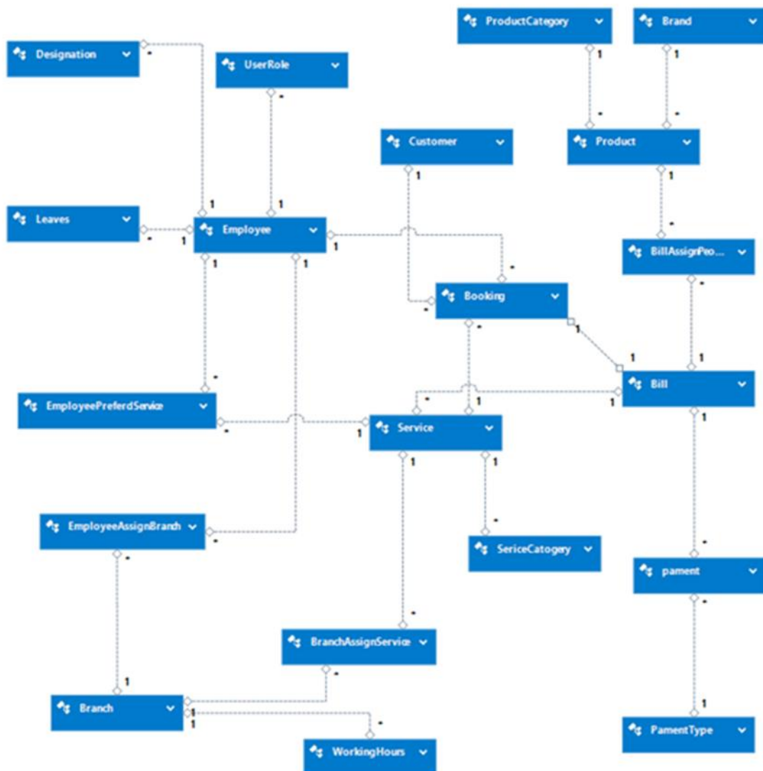
Figure 3.9: Entity Relationship Diagram for the System
