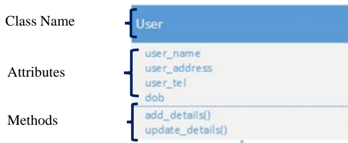
Figure 3:6 – Structure of a Class
