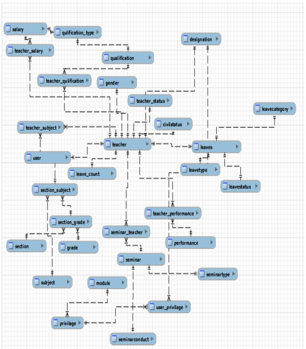
Figure 3.10 : Entity Relationship diagram for database design
