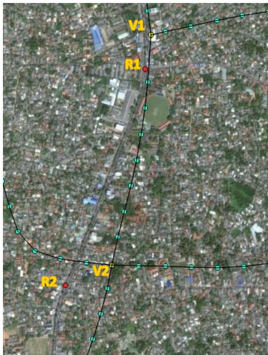
(c) R1, R2 Control points of the real road in the satellite image (shown in red color) and V1, V2 control points of the vector layer (shown in yellow).
